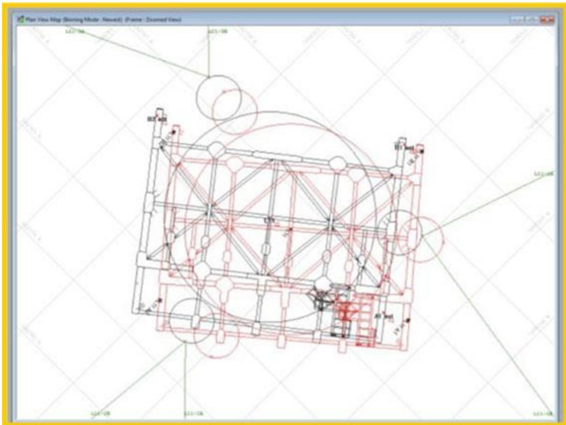
The Trimble HYDROpro screen depicts the caisson actual position in black with the required design position in red. Winch lines are also drawn on the display to help the operator determine which winches to use to move the caisson.
